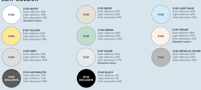
\*Please consider on south-facing elevations the high solar heat gain during the summer months may result in the glass being too warm to touch. In this case, we recommend a high solar control glass type such as SKN 176 which will reduce but not eradicate the heat. Please bare this in mind when choosing the colour of your Uni-Blinds® especially S159 and B160.
