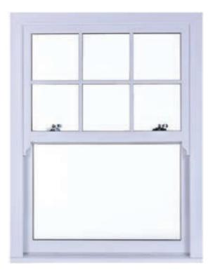
Profile detail: sculptured Meeting rail: 60mm Run through horn: flat (option) Seahorse horn: not available No horn: option Corner detail: welded Deep bottom rail: option Deep cill: not available Astragal bars: geo Furniture: acorn Removable staff bead: not available Chamber cover: not available Part Q/PAS24/SBD: option
