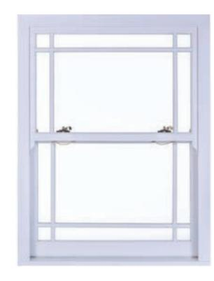
Profile detail: putty line Meeting rail: 44mm Run through horn: flat (option) Seahorse horn: not available No horn: option Corner detail: welded Deep bottom rail: standard Deep cill: not available Astragal bars: heritage Furniture: acorn Removable staff bead: not available Chamber cover: not available Part Q/PAS24/SBD: option
