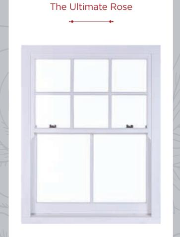
Profile detail: putty line Meeting rail: 35mm seamless Run through horn: seamless Seahorse horn: option No Horn: seamless (option) Corner detail: true mechanical Deep bottom rail: standard Deep cill: option Astragal bars: authentic Furniture: globe Removable staff bead: option Chamber cover: option Part Q/PAS24/SBD: option
